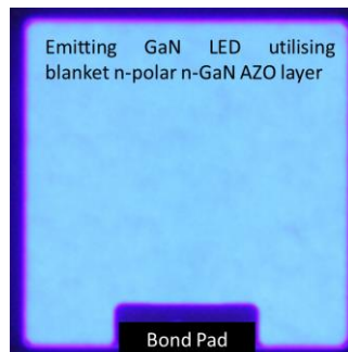
Figure 6: Optical picture of emitting MOCVD GaN LED with blanket TCO electrical contact.
