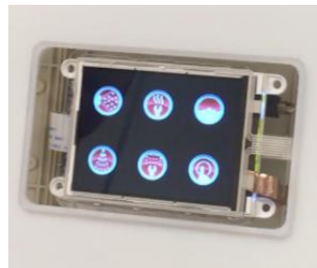
Figure 5: Working touch screen demonstrator by Quad industries utilising TCO.
